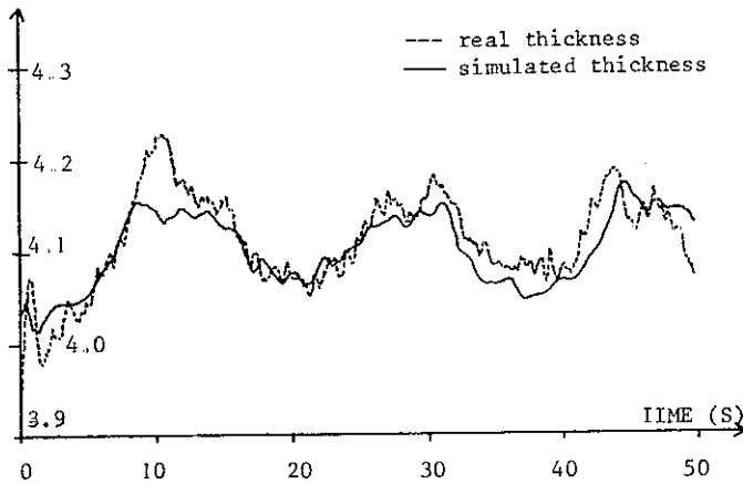
Figure 1 : Comparizon between the exit thickness obtained by the simulation and the real exit thickness
